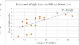
Figure 4: Correlation plot comparing the measured weight loss by the validated scale and the estimated sweat loss from hDrop. Inconsistency in hDrop measurements is clear in the poor clustering and R value of the line of best fit.
